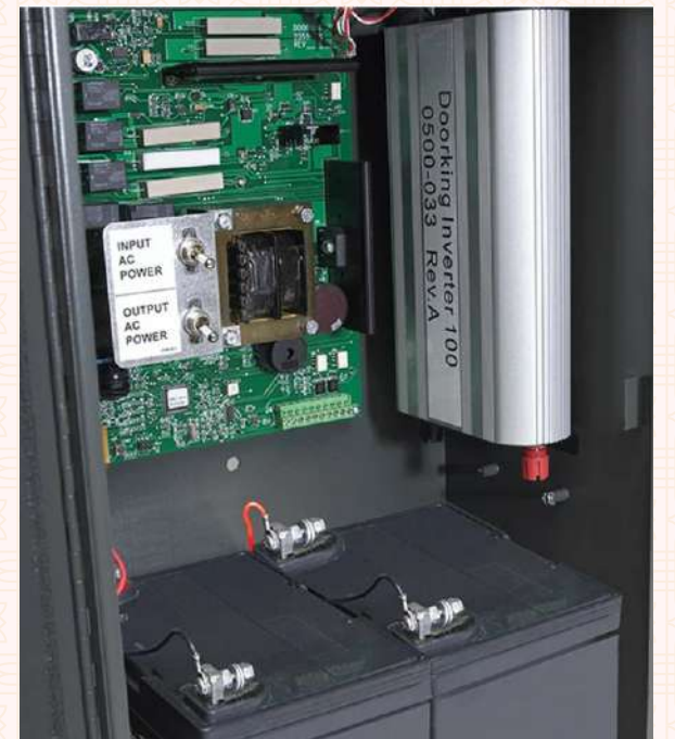
Power Backup From Inverter
